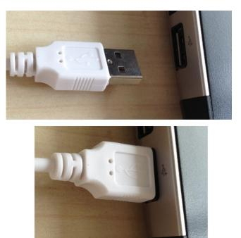
When plug the ER300D reader to the PC's USB port, the system will recognize it as HID keyboard device.
